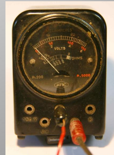
Voltmètre support bakélite Marque : Artic R = 200 ohms – 0/30 V R = 5000 ohms – 0/150 V
